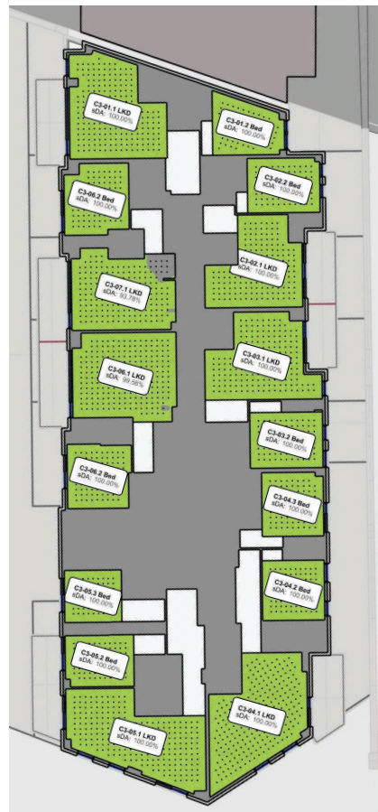
Figure 4: Floor plans indicating Daylight Provision to BS EN17037:2021+A1 Table NA.1
