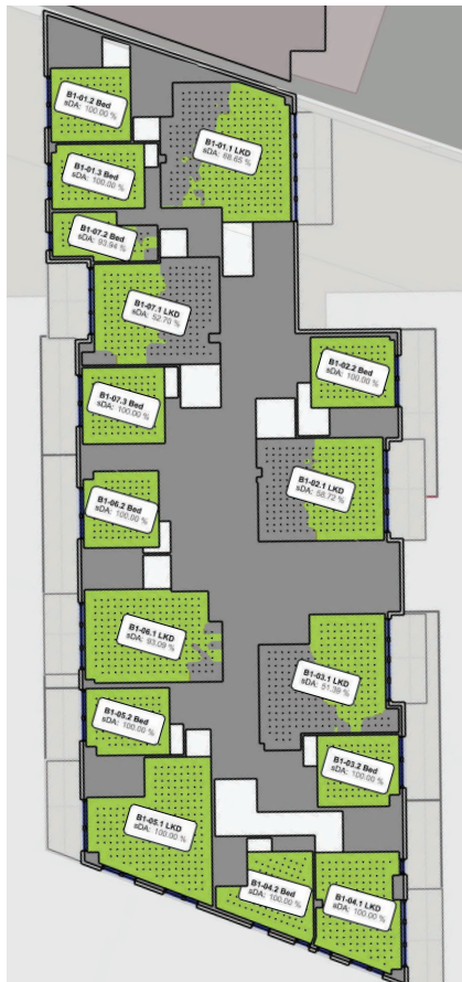
Figure 3: Floor plans indicating Daylight Provision to BS EN17037:2021+A1 Table NA.1
