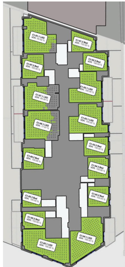
Figure 3: Floor plans indicating Daylight Provision to BS EN17037:2021+A1 Table NA.1
