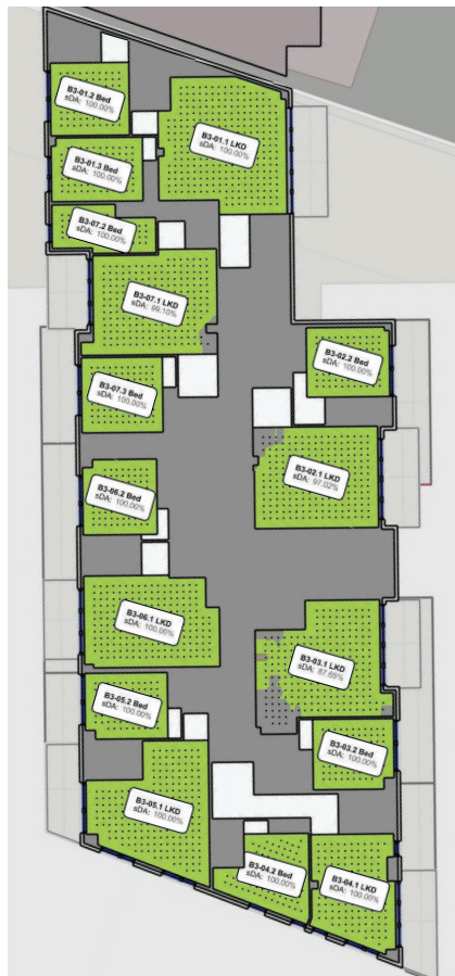
Figure 4: Floor plans indicating Daylight Provision to BS EN17037:2021+A1 Table NA.1
